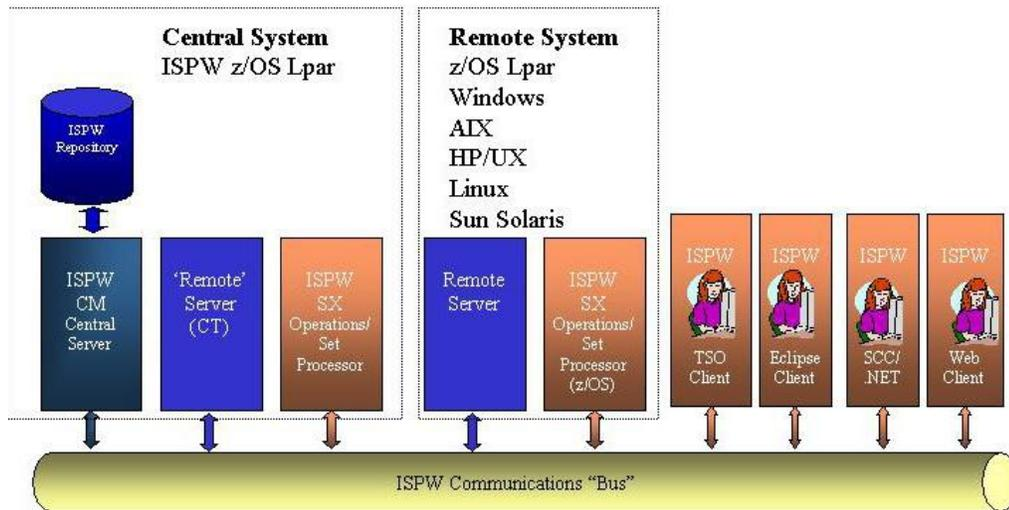
This graphic shows ISPW's modular architecture with its central server components, its remote deployment environments and its user interfaces. ISPW is a single seamless product that controls and manages application development and deployment across both the mainframe and distributed platforms.
